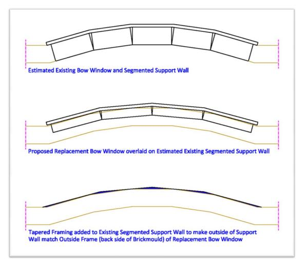
If the proposed replacement options won't work for you application, there are 2 alternate solutions, remove the protruding support wall and replace it with a protruding support wall that matches the replacement bay/bow window, or add vertical framing between the protruding support wall and the wall/roof above at the mullion locations of the existing bay and install separate rectangular windows to simulate the look of a bay or bow window.
