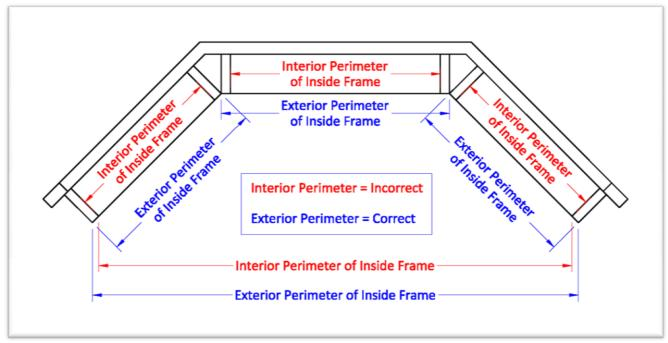
Note that this could also be measured based on the existing window jamb extension, instead of the window frame, but still needs to follow the same layout for measuring meaning follow the outside perimeter of the existing jamb extension.
