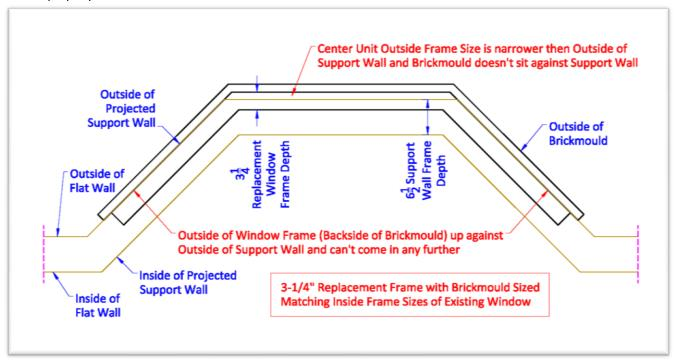
Note that if ordering the replacement bay/bow with PVC Jamb Extension at the same frame depth as the existing frame, the inside and outside sizes would both match and we won't have to adjust for any frame depth differences.
