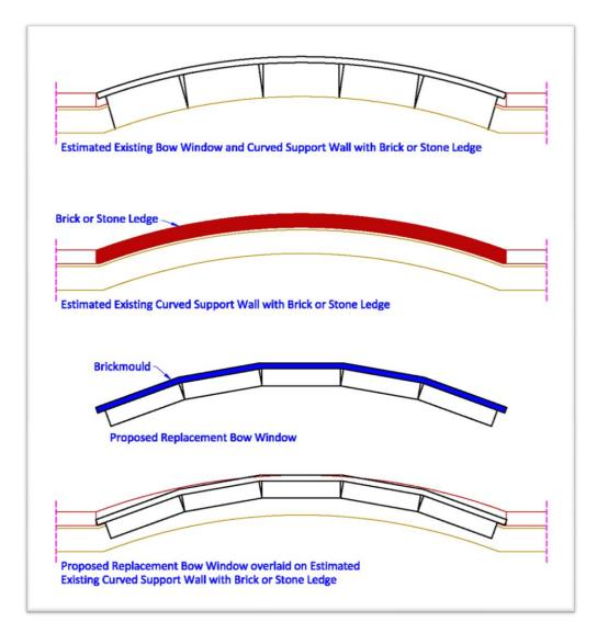
Note that the interior of the support wall won't match the replacement bow window frame. In this case we recommend ordering the replacement bow without PVC Jamb Extension so it can be custom made onsite to work with the replacement window and the inside of protruding support wall. If the replacement bow will have a head & seat board, we wouldn't need to match the interior of the protruding support wall and would only need to match the flat wall depth so the interior difference shouldn't be seen.
