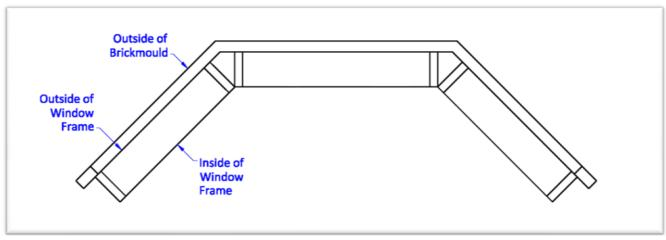
This diagram shows the bay window overlaid on the support wall, showing how the outside of the window frame (backside of the brickmould) aligns with the outside of the support wall:
